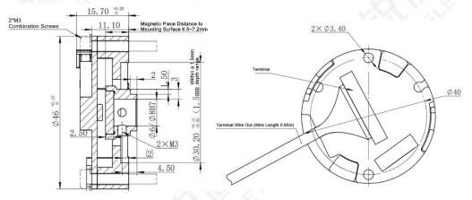
$\cdot$  Distance between the magnetic piece and the magnetic induction chip is 0.55~1.3mm
