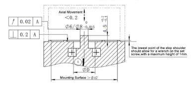
\* The lower end of the encoder shaft will be sunk into the motor end cover. When the shaft is Φ6, ΦD needs to be greater than Φ12.5; when the shaft is Φ8, ΦD needs to be greater than Φ14.5
